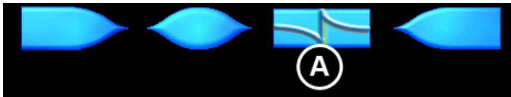
Figure 19-7: All Pass Filter
