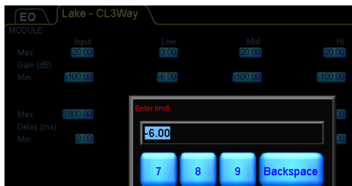
Figure 19-8: Restricting the Minimum Gain Value for Output 1
