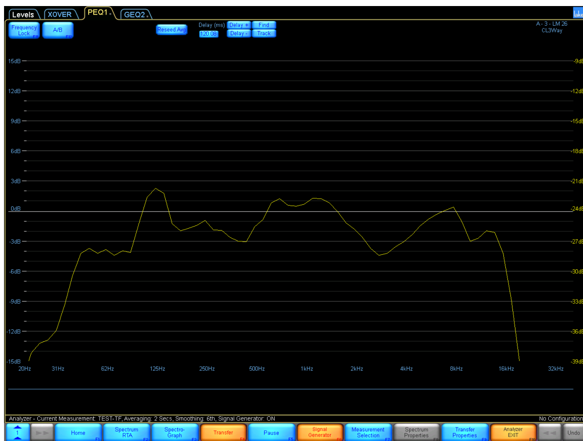
Figure 18-12: Transfer function measurement mode
