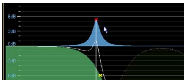
Figure 4-50: Adding a Parametric EQ to the low channel
