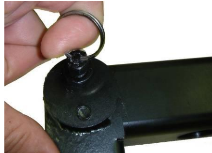
(2) Release pivoting arm locking pin
