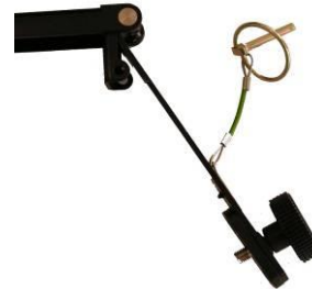
(2) Remove locking pin on the pivoting arm
